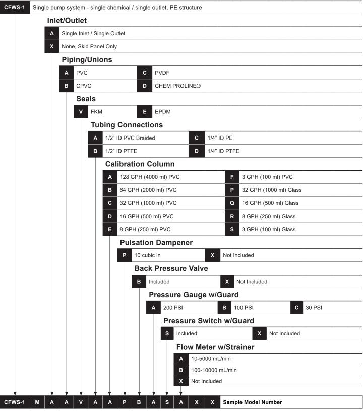
**NOTES:** When ordering pumps for skids, pump head orientation is standard LEFT facing only. Terminal Boxes quoted and mounted separately. All skids are pressure tested prior to shipment. Pumps are puchased and shipped separately. Contact factory for quote/pricing on 5-point performance testing. **Reference Adapter Kits Sheet 85000-198 when ordering with pumps utilizing "M = 1/2"MNPT" or "F = 1/2"FNPT" connections.**
