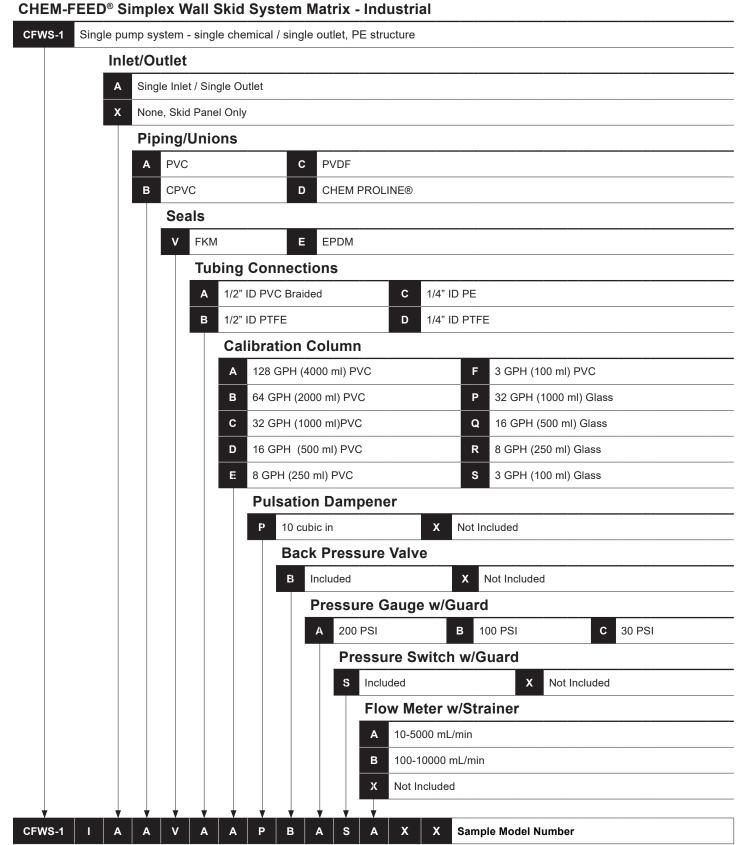
**NOTES:** When ordering pumps for skids, pump head orientation is standard LEFT facing only. Terminal Boxes quoted and mounted separately. All skids are pressure tested prior to shipment. Pumps are puchased and shipped separately. Contact factory for quote/pricing on 5-point performance testing. Reference Adapter Kits Sheet 85000-198 when ordering with pumps utilizing "M = 1/2"MNPT " or "F = 1/2"FNPT" connections.
