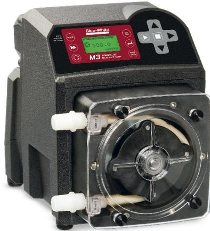
The FLEXFLO® M3 is equipped with Blue-White's exclusive, built-in, Tube Failure Detection System (TFD). This technology detects a wide range of conductive chemicals with no false triggering. If the TFD detects tube failure, the pump will automatically shut off and energize a relay switch. This permits communication with external equipment, such as a back-up pump or alarm. It also serves to prevent chemical spills and added downtime.
