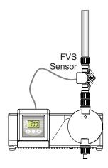
**Confirm FVS flow range -** Flow Verification Sensor (FVS) will only function within its operating range. See chart for available ranges.
