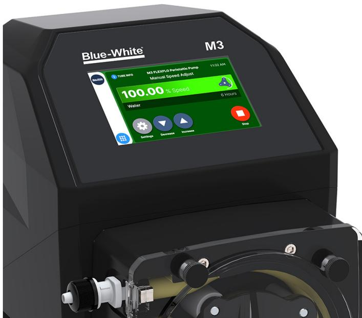
**Calibration.** Chemical metering systems should be calibrated at the initial start-up as well as after maintenance has been performed (e.g., when a tube is changed in a peristaltic pump). If the metering pump does not have an internal calibration process, operators can use a calibration cylinder and do a drawdown to check how much fluid is being pumped at a given setting. Other times, the pump can be tied to an external device such as the flow meter, which can pace the pump's output.
